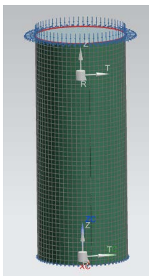
Figure 4 Tube test FEA setup
