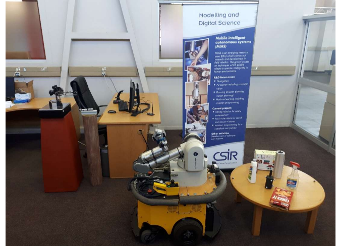
Figure 12 The kinaesthetic teaching setup.
