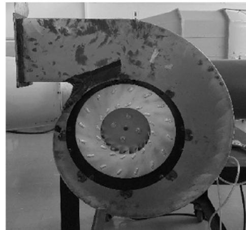
Figure 5 Open impeller and volute
