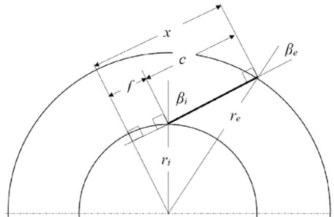
Figure 1 The geometry of impellers with straight, back-swept blades
