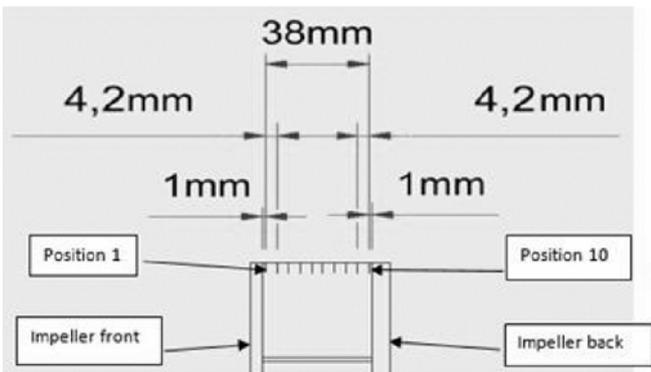
Figure 8 Diagram of measuring positions across impeller width
