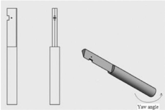
Figure 7 Wedge probe
