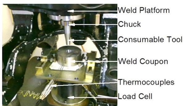
Figure 4 Weld and Experimental Set Up
