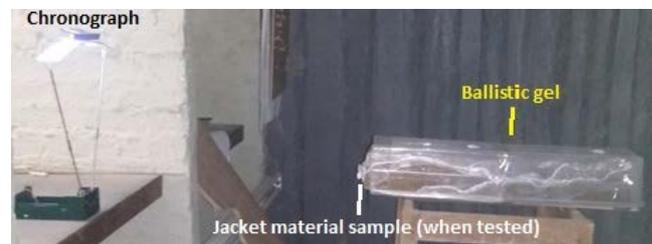
Figure 1 Side view of the equipment setup.
