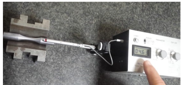
Figure 7 Surface roughness measurement being conducted on the fatigue test specimen.
