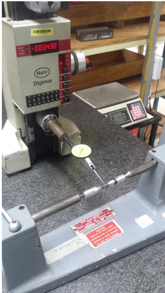
Figure 5 Measurement of eccentricity of the specimens.
