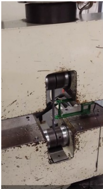
Figure 8 Static test specimen in the test machine.
