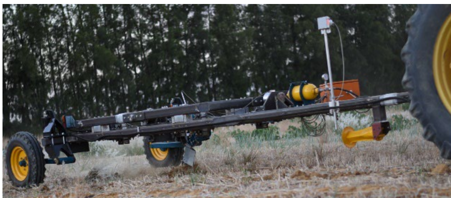
Figure 16 Action photo of the test setup being pulled by a tractor during in-field testing of the tine ripper unit.
